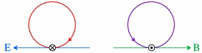
Figure 2. Axial view of the circuit, showing positronic WSGB propagating into the page and electronic WSGB propagating out of the page.
